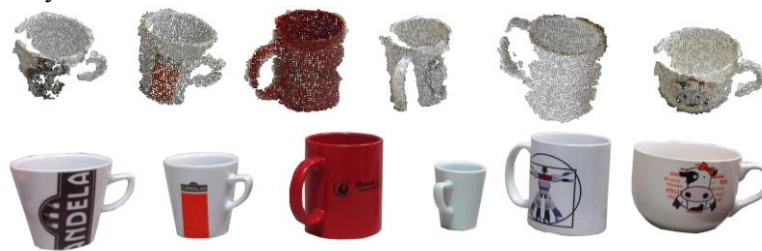
Fig. 4. 3D and color representations for the different objects that form the database. Notice that most of the items are geometrically similar.
