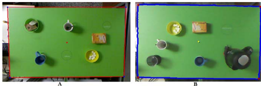
Fig. 3. Comparison of vision-based techniques for table detection. A) Depth-based algorithm; B) Color-based algorithm.
