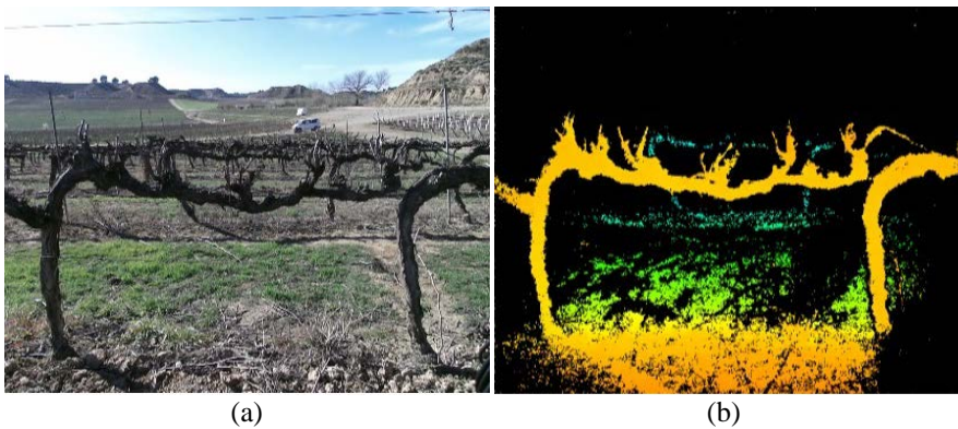
Fig. 3. (a) Color image taken by Kinect v2 sensor (b) Depth image taken by Kinect v2 sensor.
