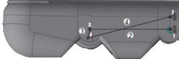
Fig. 2. Four-bar linkage in the interphalangeal joints.
