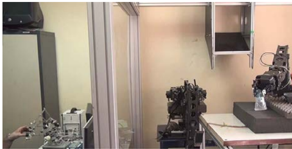
Fig. 4. A user performing the dexterous teleoperation task with the 3-Finger Haptic Device.
