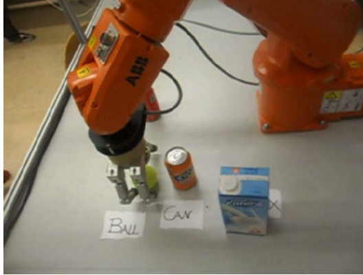
Fig. 2. Object sorting: Different objects are shown once the robot has sorted them
